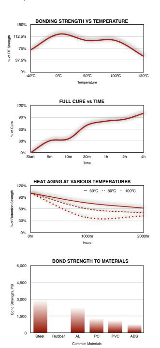
Figures are tested to ASTM 4501. Results may differ with varying application bonding areas, contact surface areas, coatings and
