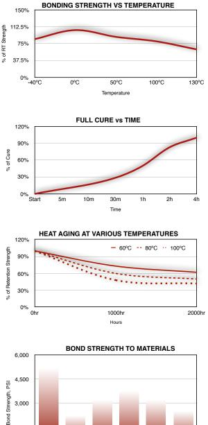
1,500 0 Steel Rubber AL PC PVC ABS Common Materials Figures are tested to ASTM 4501. Results may differ with varying
