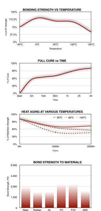
Common Materials Figures are tested to ASTM 4501. Results may differ with varying application bonding areas, contact surface areas, coatings and material grades, etc.
